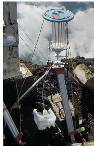
Fig. 1 Passive-type fog sampler at the top of Mt. Fuji
