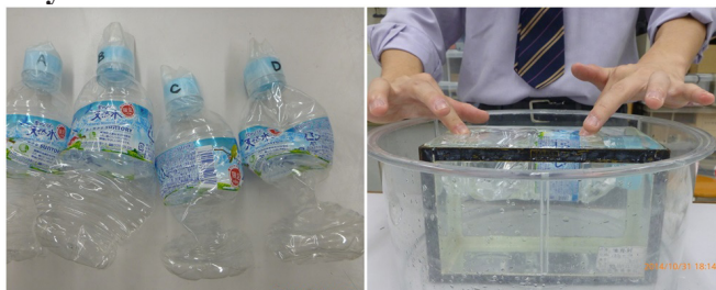
PET bottles closed at MFRS and brought down to measure the volume
