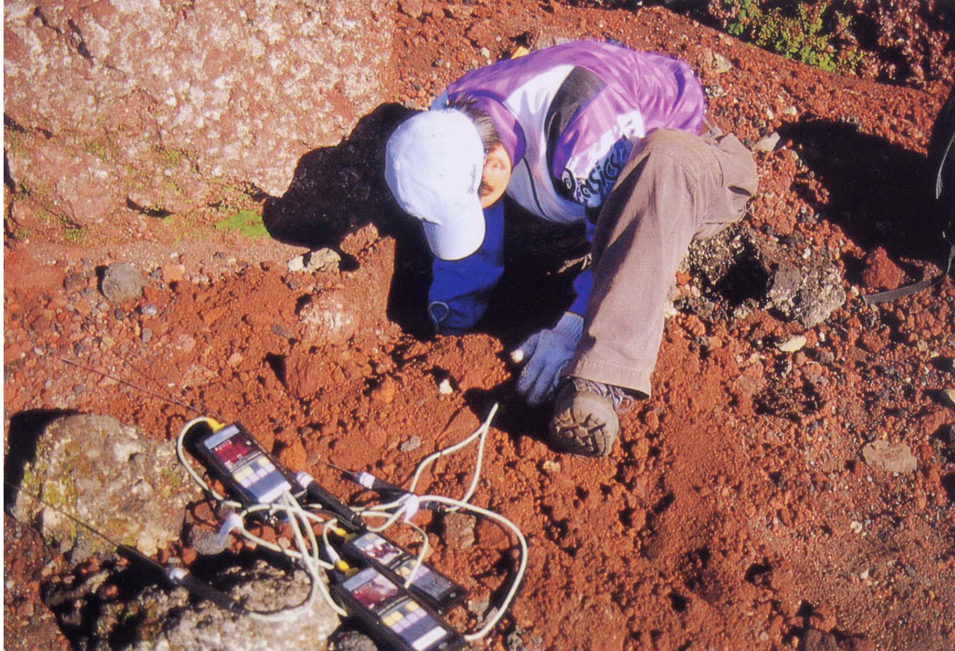
The depth to the permafrost was measured by data logger with long rod sensor.
